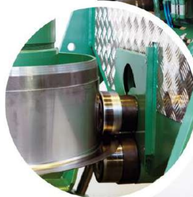
Flanging unit after completed operation
