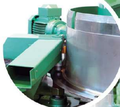
Punching of holes in the flange
