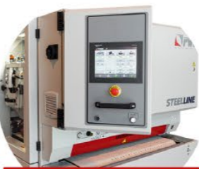
TILTING CONTROL PANEL
