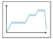
In case of a fall, the tearing of the energy absorber webbing limits the impact force on the user. The lanyards are designed for users who weigh between 50 and 130 kg. The progressive tearing of the webbing reduces the deceleration on lightweight users.
