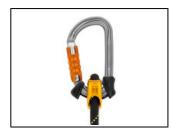
The CAPTIV ADJUST positioning bar promotes loading of the carabiner on the major axis and helps hold the ADJUST rope adjuster in the proper position to reduce the risk of accidental release.
