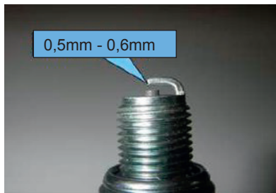
Fig. 30: Electrode gap of the spark plug
