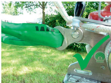
Fig. 22: Correct fastening the EDER Powerwinch 500
