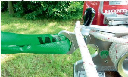
Fig. 20: Guiding the rope through the clamp
