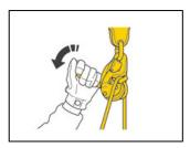
Evacuation with the I'D EVAC descender, whose ergonomic handle allows the user to easily control the rope's descent speed during evacuation.
