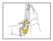
The ROLLCLIP A pulley may be used as a directional point on the lower attachment point of the ASCENSION handled rope clamp, for short rope ascents. Gate opening on the pulley side facilitates installation of the rope.
