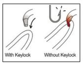
To ensure optimal efficiency, Sm'D carabiners use the Keylock system: the body/gate interface does not have a hook that could snag on anchors, ropes, harness equipment loops...
