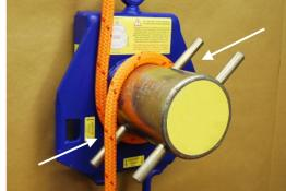
(1) Ensure the working line enters the device from a (4) vertical point directly above the device.
