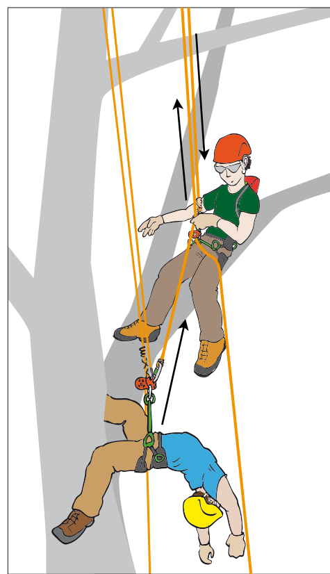
Termination of climbing line attached to injured climber. Rescuer descends on add-in prusik
