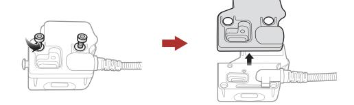
3. Remove the rubber pad and replace it with the thicker rubber pad included in the package.
