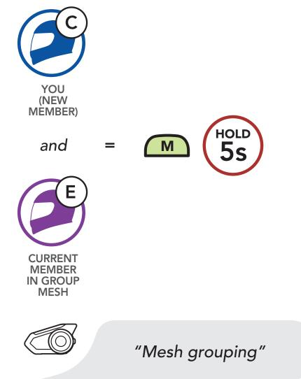
2. The headsets complete **Mesh Grouping**. The new members will hear a voice prompt as their headsets automatically switch from Open Mesh to Group Mesh.
