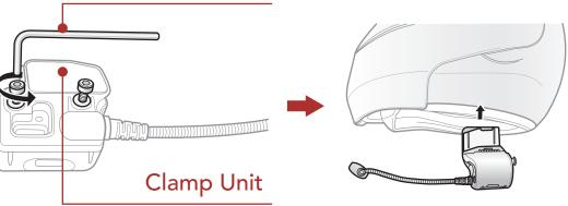
**Note:** Depending on the size and shape of your helmet, you may need to change the thickness of the rubber pad between the clamp plates using the two extra rubber pads in the box. To increase the overall thickness, attach the thinner one to the original rubber pad or replace the original rubber pad with the thicker one.
