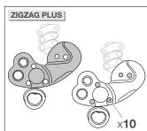
• On pre-2019 ZIGZAG, check for wear at the points where the friction chain stops against the frame. Look for sharp edges that could damage your rope. If necessary, round any sharp edges with fine-grain sandpaper.
