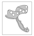
• Check the articulation between the handle and the frame, and the effectiveness of the return spring.
