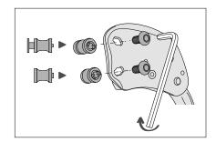
• Check the condition of the opening buttons (marks, wear, dirt), and verify that the moving side plate closes properly.
