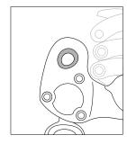
• Check the edges of the attachment hole for wear caused by the connector.
