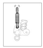
• Check the condition of the positioning ring (deformation, cracks, cuts...).
