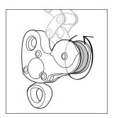
• On pre-2019 ZIGZAG and on the ZIGZAG PLUS, check the condition of the swivel (cracks, deformation...).
