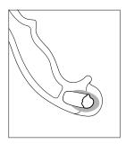
• Check the tightness and condition of the friction pins (wear, deformation, corrosion). Rotate or replace the pins if necessary.
