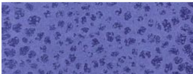
Close-up image of phase separation on flat surface. PG-24 Night Rain on AMACO 30M clay. Fired to cone 5.
