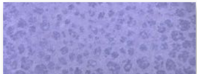
Close-up image of phase separation on flat surface. PG-55 Floating Lavender on AMACO 30M clay. Fired to cone 5.
