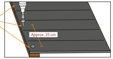
Fix the mat, lying on the floor, onto the wooden board (tensionless installation)
