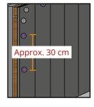
Lay a wooden board underneath and fix it in place
