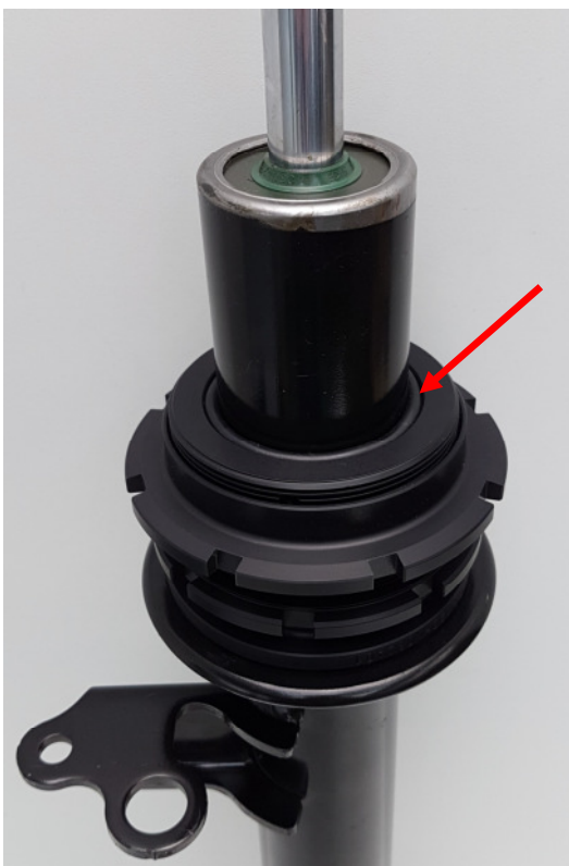
Abb. 3: O-Ring montieren (nur ohne DDC) Fig. 3: Mount the sealing ring (only without DDC)
