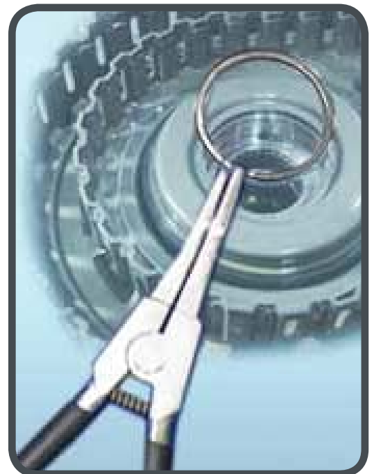
⇧ Pliers for removing/installing the safety ring.
