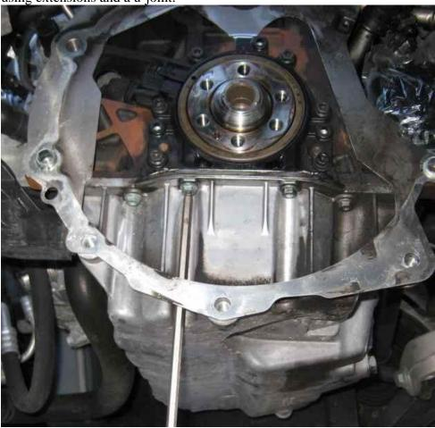
Gently pull the seal flange straight off. Don't pry close to the sealing surfaces of the crankshaft or you might scratch it.
