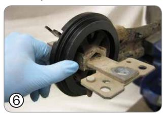
Fit **AST5114-3 Removal Adaptor Plate** over the 'T' shaped end of the bush and position it flat against the arm so that the cable stay bracket is positioned in the recess of the adaptor plate.
