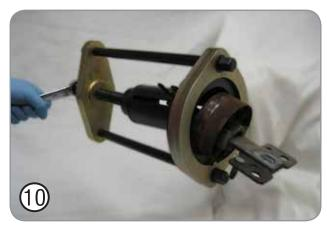
When the bush and bush tool are correctly aligned, use a 24mm spanner to tighten the Force Screw of the Bush Tool, slowly and smoothly pressing the bush out of the trailing arm.
