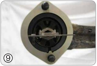
Before pressing the bush from the arm, check that the tool is correctly aligned. Misalignment of the tool may lead to the bush being pressed out at an angle, causing damage to the tool and the trailing arm.
