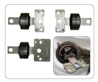
**AST5114 Trailing Arm Bush Remover/Installer Kit** is designed for **ON CAR** applications. This minimises the amount of disassembly required, significantly reducing the length of time taken to replace the bushes.
