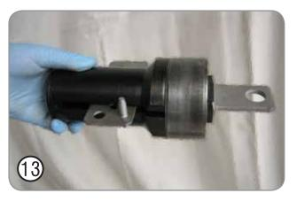
Position the replacement bush in the slot of **AST5114-2 Thrust Tube**, locating the outer sleeve of the bush onto the end face of the Thrust Tube.
