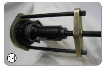
Position **AST5114-2 Thrust Tube** and the replacement bush in the Frame. Then tighten the force screw **hand tight only** at this stage, so that the frame and bush are retained in position, but the bush is not forced into the arm.
