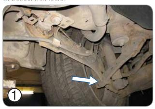
Remove the bottom bolt of the shock absorber and the support link bar bolt from the trailing arm.
