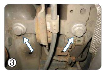
Remove the 2 bolts that secure the front end of the trailing arm to the underside of the vehicle.
