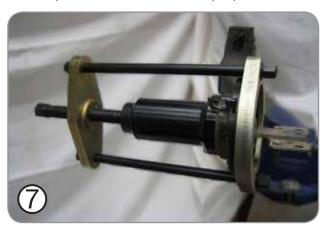
Fit AST5114-1 Frame assembly over the bush and trailing arm, then position it so that the lug of the frame bottom plate is located in the slot of AST5114-3 removal adaptor plate. Fit AST5114-2 Thrust Tube over the trailing arm bush and tighten the force screw hand tight only at this stage, so that the frame is retained in position, but not forcing the bush from the arm.
