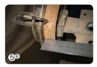
Before removing the trailing arm bush, take note of the position of the bush, including the distance that the outer sleeve of the bush protrudes from the outside of the trailing arm.
