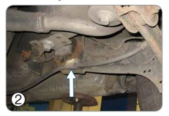
Unclip the cables and the electrical wiring from the trailing arm, detach the bracket that is bolted to the trailing arm bush.
