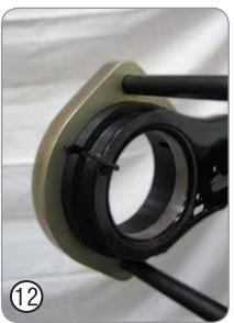
Fit the assembled Frame and Adaptor Plate over the trailing arm, locating the cable stay bracket into the slot of the installation adaptor plate. This will position the frame at the correct angle for installation of the bush.
