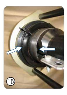
Check that the Bush, Trailing Arm and Frame assembly are correctly aligned. The rubber lua moulded into the bush should align with the cut out at the end of the trailing arm (or paint marks if used). The Force Screw, Thrust Tube and Central bar of the bush must all be aligned to ensure that the bush is pressed into the trailing arm correctly.
