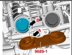
Insert camshaft retainer (9689-1) into camshaft openings until stop.
