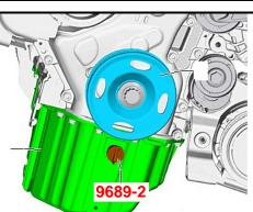
Place the pointer (9689-2), vertically aligned and pointing upwards, into the hole in the oil pan.
