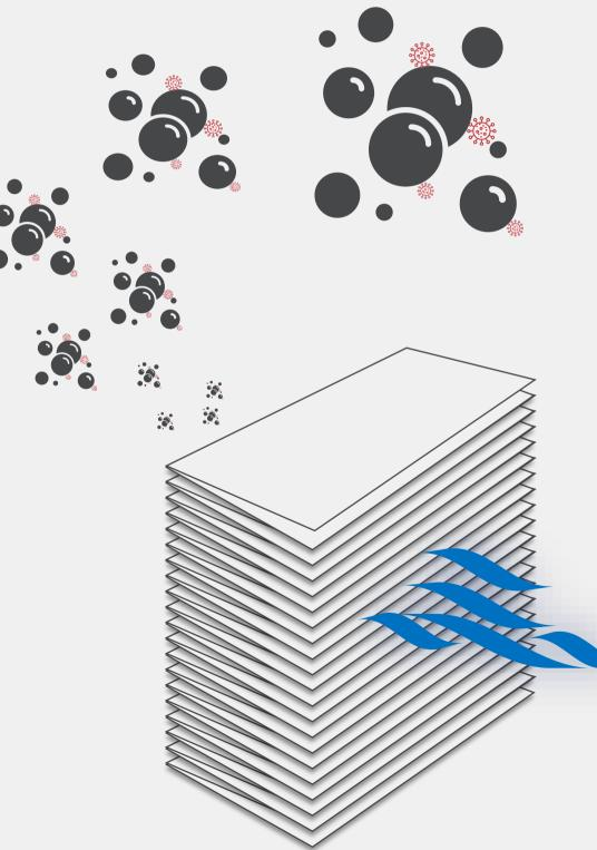
In general: The minimum deposition (or maximum penetration) of particles in HEPA filters is in the size range of around 0,1-0,2 µm for glass media, for ePTFE/eFRM it's a little bit below. Towards smaller particles as well as towards larger particles the deposition is larger!
