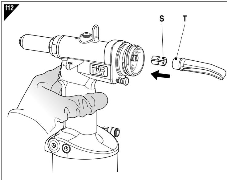
In case you want to convey the pieces of sheared nails inside a container, pull out the baffle (T) and the relative reduction (S) from the tool.
