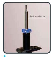
6. Remove the rod-puller after locking the clamp in its final configuration.
