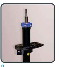
1. Position the clamp with the fixing screws. DO NOT TIGHTEN.
