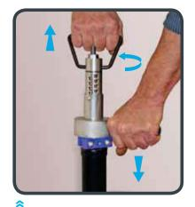
3. Remove the stem puller and lock it with a slight rotation to the right or left. **NB**: it is possible to extract the stem by another 20 mm keeping the support still and turning the stem puller.
