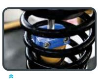
7. Mount the spring and remove the clamp.
