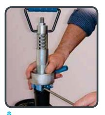
4. When the removal is completed, lock the clamp with the screws.
