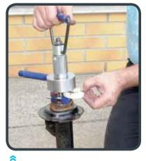
5. If rod-puller stroke is insufficient: insert one or both spacers (provided) between the support and the clamp in order to further extract the shock absorber rod.
