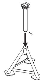
3. Make sure that the ratchet bar is secured and can not be lifted out of the stand.
