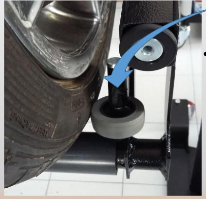
Thanks to the little rubber wheels, the <u>wheel rims</u> won't be scratched and will be protected from damage
