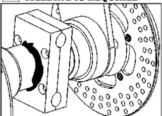
Before Welding: make sure the axle assembly is properly aligned with the transmission is properly aligned with the transmission drive pulley, and the belt or chain clears the windows on housing, if the belt/chain does not clear the windows serious damage may occur to housing and may result serious injury to the rider.
