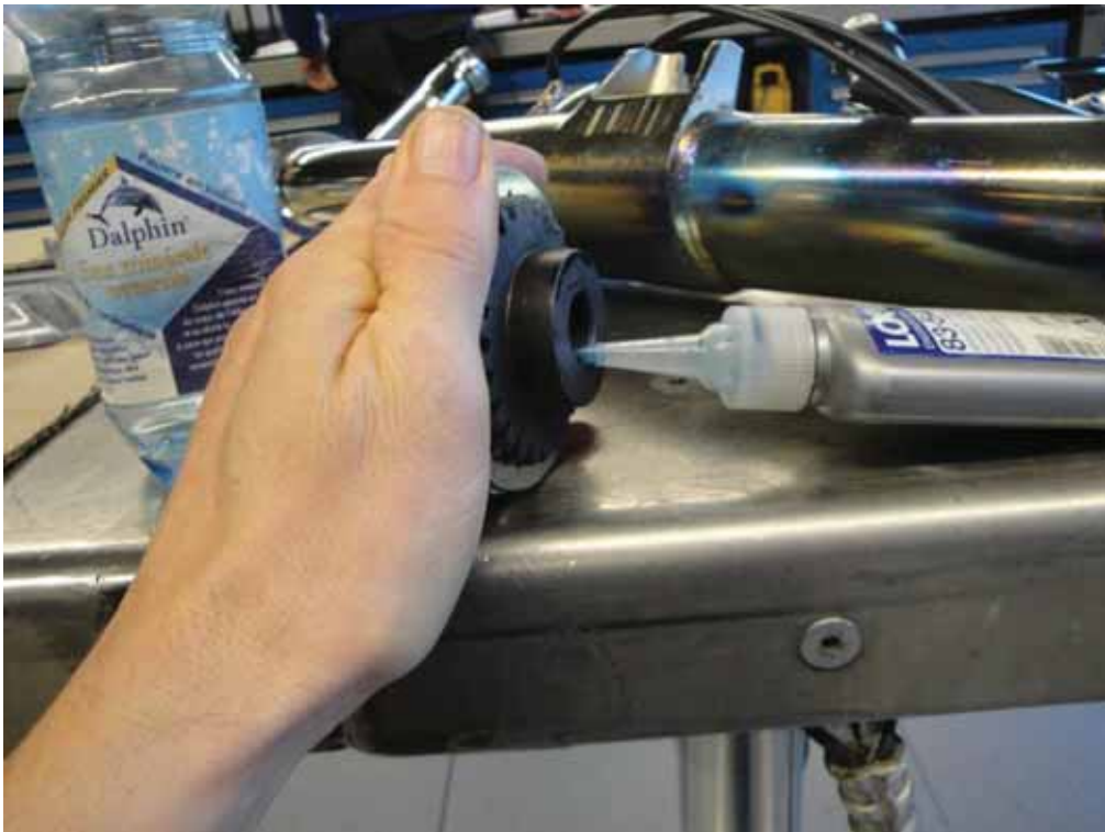
Mount the sprocket with strong Loctite.
