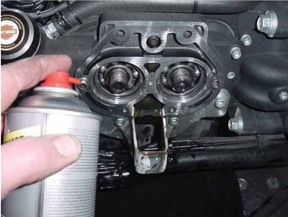
Clean the screw-thread with brake cleaner.
