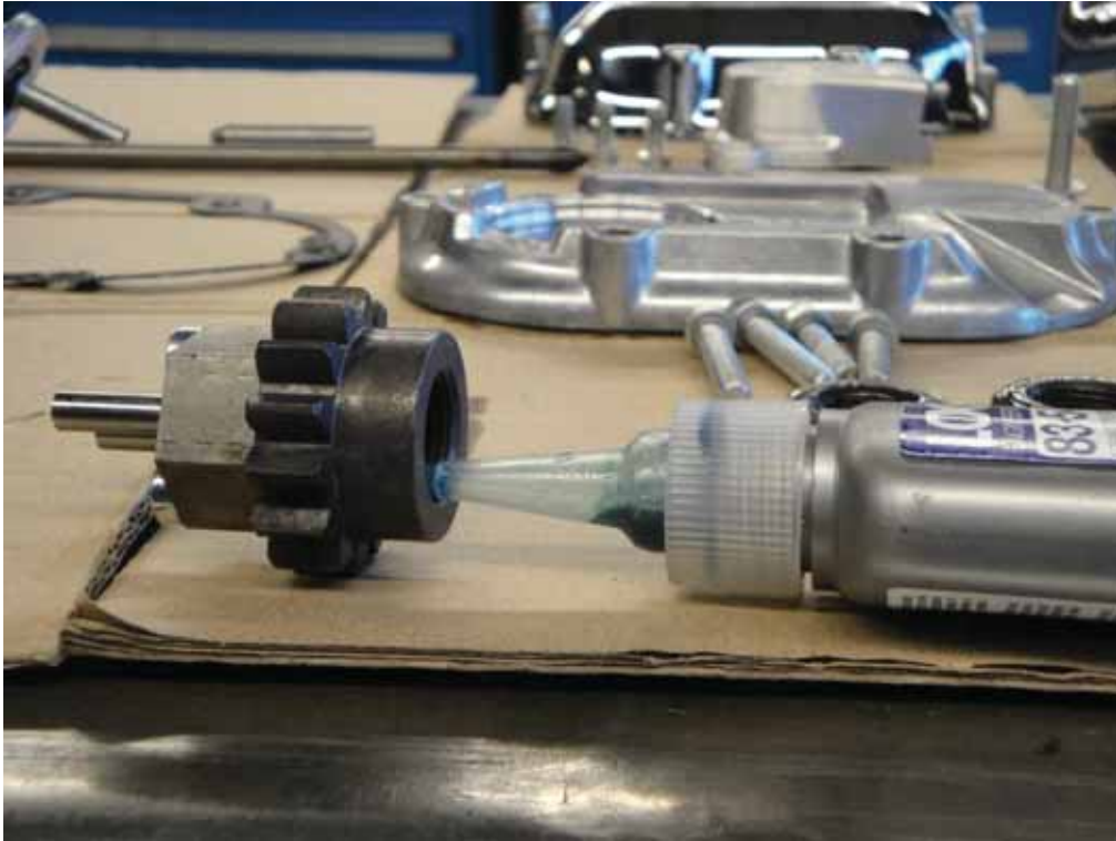
Mount the sprocket with strong Loctite.
