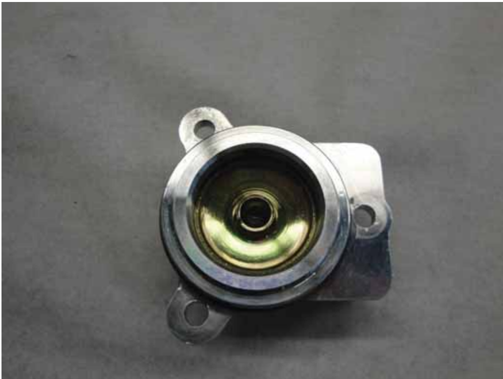
Remove the piston of the hydraulic operated clutch cilinder.
