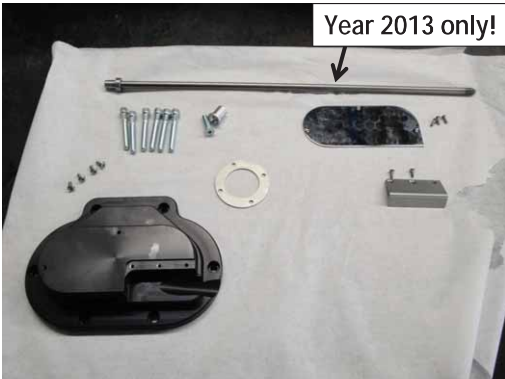
Hydraulic clutch cylinder housing kit. Only necessary if the bike is fitted with an hydraulic clutch. The additional pushing rod is only necessary in 2013 models.
