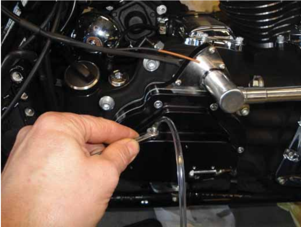
Mount the bleed nipple and bleed the clutch.
