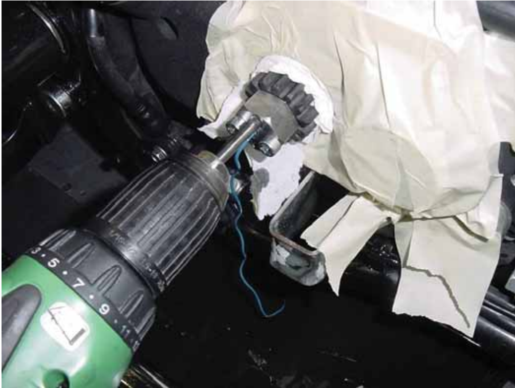
Mill the two holes shown in the pictures.
