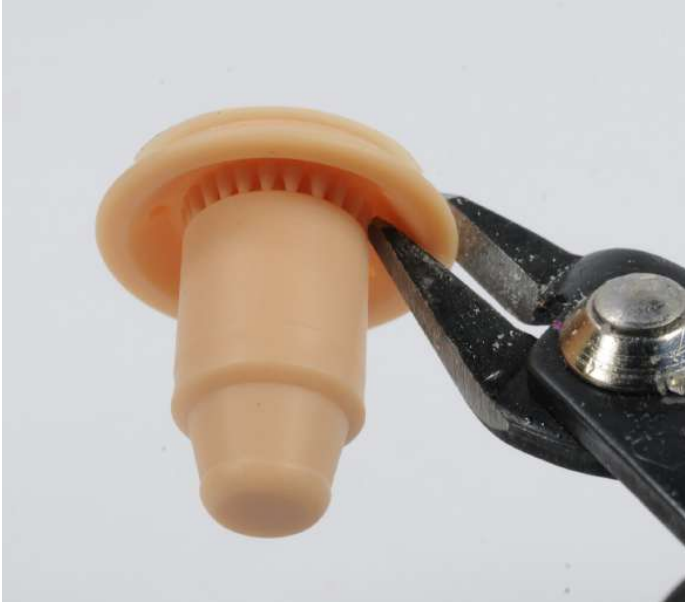
3Shape only: Remove supports inside insertion holes
