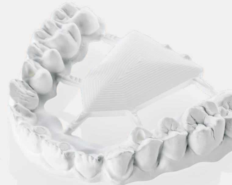
The number of connectors between the sintering block and the bridge should be at least four.
