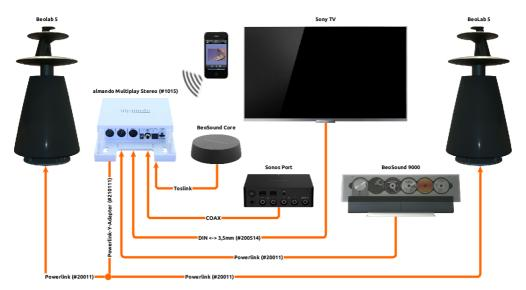
Powerlink signals from connected B&O devices are simply looped through. All other audio signals - whether digital or analog - are converted to a 100% standard B&O Powerlink signal including the trigger voltage required for the B&O loudspeakers (as well as the B&O data signal for BeoLab 5, BeoLab 4500 and BeoLab Penta if required).
