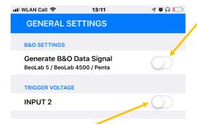
Here you determine whether data signals will be sent to the B&O speakers (input data from connected B&O devices or data generated by the almando Decoder itself for third-party devices). This is only necessary if BeoLab 5, BeoLab 4500 or BeoLab Penta are connected. Otherwise the generation of the "data signal" should remain deactivated (default setting).
