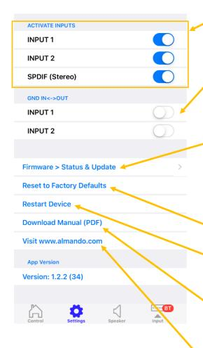
If no devices are connected to certain inputs, they can be deactivated here. They will then be hidden on the main screen of the app. This setting can be undone later at any time.
