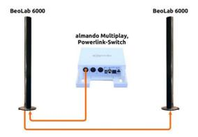
If your B&O speakers each have two Powerlink sockets, you can also loop the Powerlink cables through (daisy chain) - from one speaker to the next, like a chain of lights.
