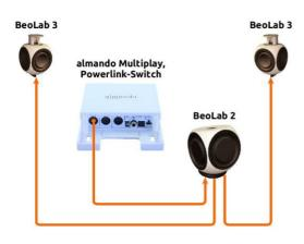
You can also connect a subwoofer. The subwoofer itself has two further Powerlink sockets to which you connect the pair of speakers.
