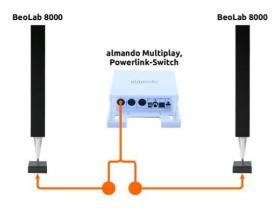
To connect your B&O speakers individually, you need a Powerlink-Y-Adapter (#210111), because the almando Multiplay and the almando Powerlink-Switch have only one output socket.
