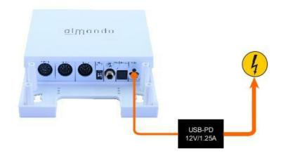
Once you have installed the app on your smartphone or tablet, connect the almando Multiplay Stereo or the almando Powerlink switch to the mains using the USB power adapter.
