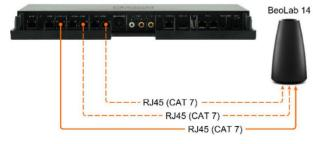
BeoLab 14 can also be easily connected here (center and subwoofer are output separately on both audio signals from the Powerlink socket).
