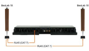
If the speaker has two Powerlink sockets, looping through is also possible (daisy chain).
