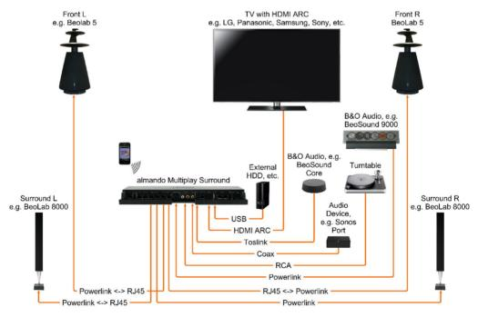
The almando Multiplay Surround can be individually configured using a smartphone app. This allows you to set all parameters such as lipsync, downmix, Pro Logic mode, volumes and distances of the speakers and make sound settings such as treble, bass and loudness, etc. And sometimes even individually for each input. This means you can tailor your surround setup perfectly to your needs.
