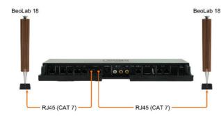
Newer B&O speakers (e.g BeoLab 18) connect directly with a CAT 7 patch cable.
