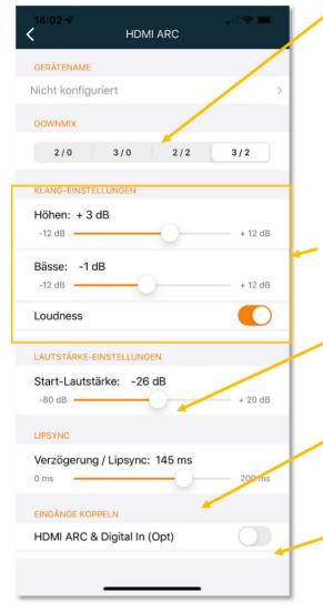
In the DOWNMIX area you determine which speakers should playback when this input is active. The first number means the number of front speakers. The number after the slash indicates the number of rear speakers. For example, when watching TV, you can play the sound in full surround sound (HDMI: 3/2) and, on the other hand, only have your B&O system run in stereo via the two front speakers (DIN: 2/0).
