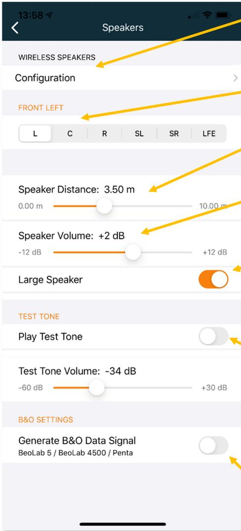
Optional: If the device has an integrated WiSA transmitter module you can open a page to connect wireless speaker (e.g. BeoLab 18).
