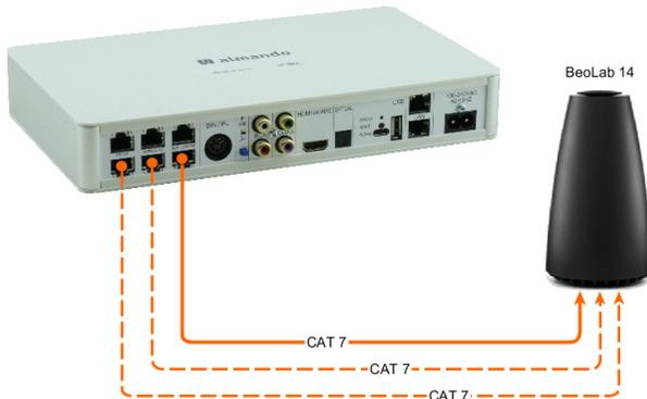
BeoLab 14 can also be connected without any problems (center and subwoofer channels are separately on both audio signals of this Powerlink socket).
