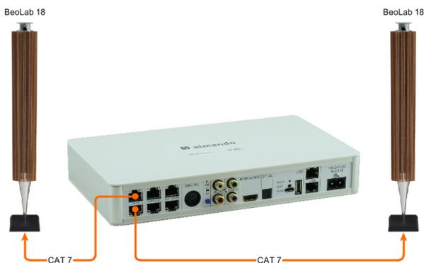
Newer B&O speakers (e.g., BeoLab 18) will be connect directly with a CAT 7 patch cable.
