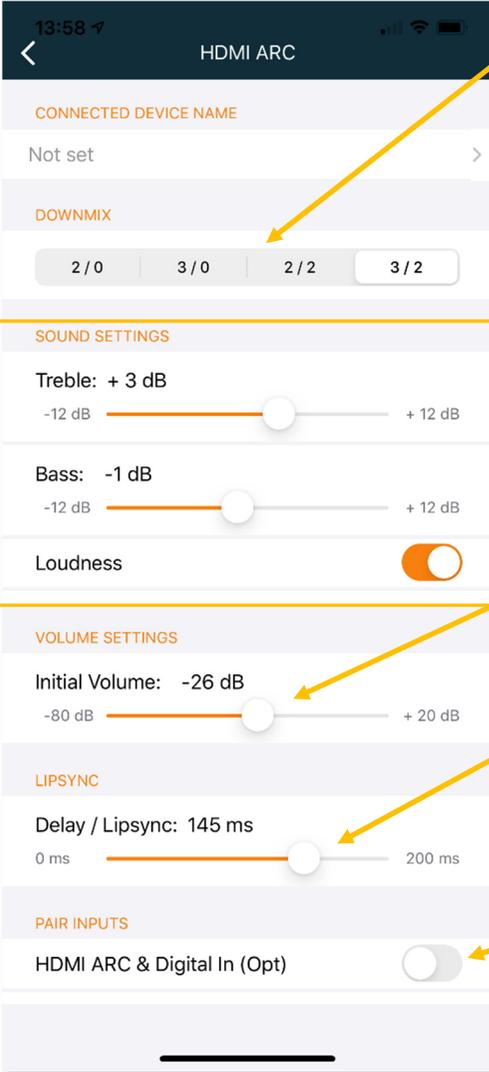
In the area of DOWNMIX you can determine on which speakers the playback should take place, if this input is active. The first number means the number of front speakers. The number after the slash indicates the number of rear speakers. So you can, for example, when watching TV, play the sound in full surround sound (HDMI: 3/2) and in contrast, let your audio device run in stereo only via the two front speakers (DIN: 2/0).
