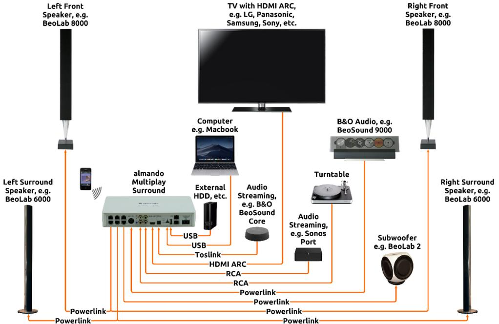
The almando Multiplay Surround can be individually configured with a smartphone app. This allows you to set all parameters such as Lipsync, Downmix, Pro Logic Mode, volume and distances of the speakers, and adjust the sound settings such as treble, bass and loudness, etc. And all of this is even partial for each input individually. This allows you to set up your surround system to your needs.
