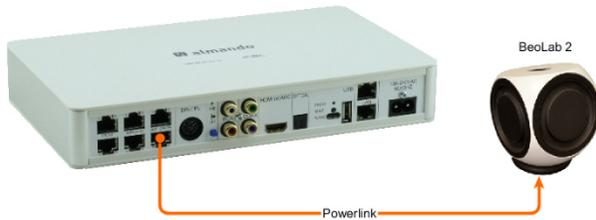
Subwoofers like a BeoLab 2 are connected to the lower right RJ45 socket.
