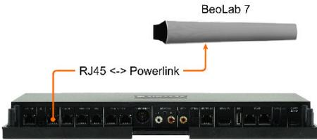
Both mono and stereo speakers (as shown here, a BeoLab 7) can be connected to the center socket. The center tone is output here on both Powerlink audio signals of the socket.
