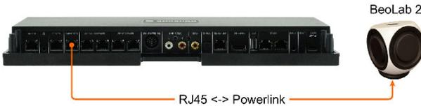
Subwoofers - like a BeoLab 2 shown here - are connected to the corresponding RJ45 socket.
