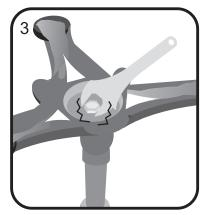
Tighten the bolt with a spanner.
