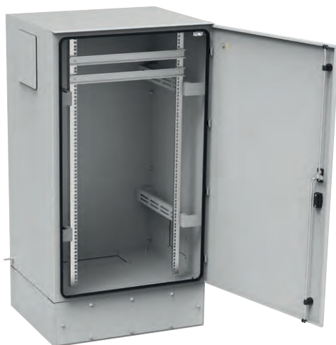
Outdoor cabinet with 19" mounting profiles body dimensions 1140 x 714 x 600 mm, protection degree IP 55, mechanical resistance IK 10, designed in three versions: free-standing (with plinth), wall-mounted or pole-mounted
