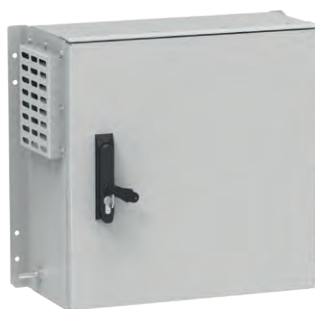
Outdoor cabinet with DIN rails body dimensions 500 x 500 x 210 mm, protection degree IP 55, mechanical resistance IK 10, designed for wall mounting
