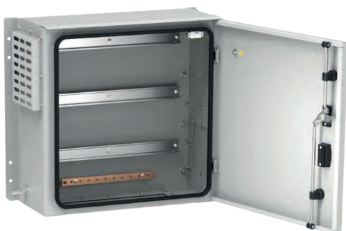
Outdoor cabinet with DIN rails body dimensions 500 x 500 x 210 mm, protection degree IP 55, mechanical resistance IK 10, designed for wall mounting
