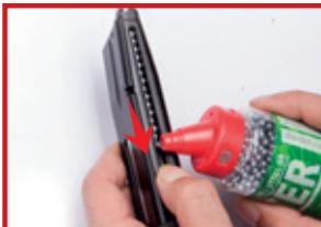
The magazine is now ready to be loaded with 4.5mm steel BBs. Remember to release the BB hatch after loading the BBs.
