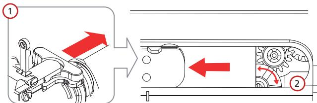
1. To adjust the Hop-up, pull the cocking lever to reveal the adjustment lever.
