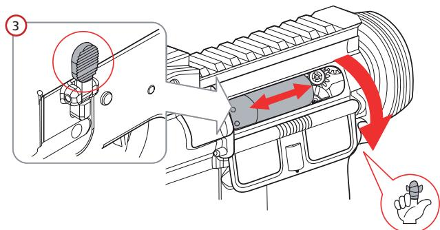
3. Push the bolt catch to release the bolt plate.
