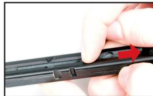
Push the magazine release button and pull out the magazine. Pull down the magazine follower.
