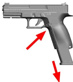
Push the magazine release button and pull out the magazine.
