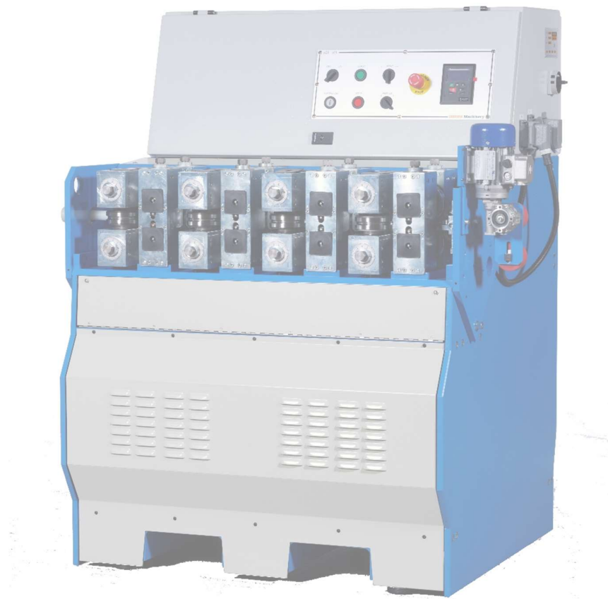
KOR-108 – Reduction rolling machine for tubular heating elements
