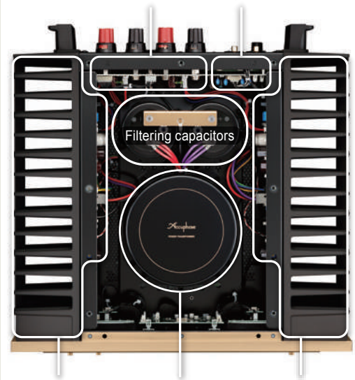
L ch power amplification section Toroidal transformer R ch power amplification section
