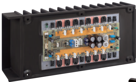
⑮ Power amplification section
