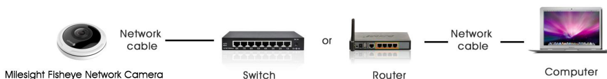
Figure 2-1-2 Connect via a switch or a Router
