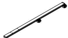
Standard post for VARIO system including pipe bracket.
