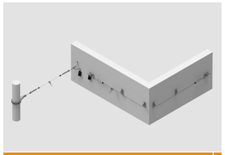
The ALLinONE lifeline system from INNOTECH has been developed for multiple fall protection systems, and is used as a restraint
