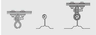
The SYST from INNOTECH can be used as a end or corner post or intermediate bracket in the horizontal lifeline system.
