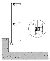
2 anchorage points are provided for installation of the spacer bracket. (Adapter on the inside of the parapet, hinged A31:  $2 \times Ø$  15 mm)
