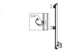
**OPTIONAL:** Height adjustment of the pipe bracket
