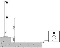
If the parapet is  $\leq$  150 mm, then a toe board is required.
