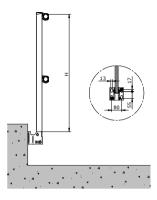
2 anchorage points are provided for installation of the spacer bracket. (Adapter on the inside of the parapet A11:  $2 \times Ø 15 \text{ mm}$ )
