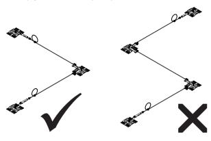
INNOTECH "SANDWICH-13" is suitable ONLY for cable spans with  ${\bf one}$  corner point.
