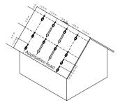
Installation configuration as pictured and according to the need for anchor points (e.g. roof exit, chimney, solar installation, etc.) or as required by local law or in accordance with DIN 4426.
