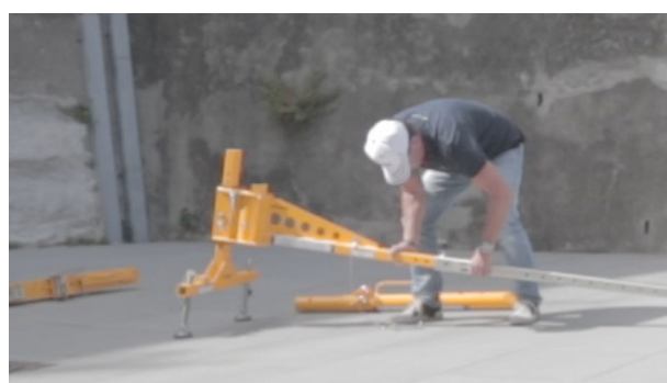
Step.4 Insert the A2126-09 extension into the IN-2126 or IN-2204 T-Base
