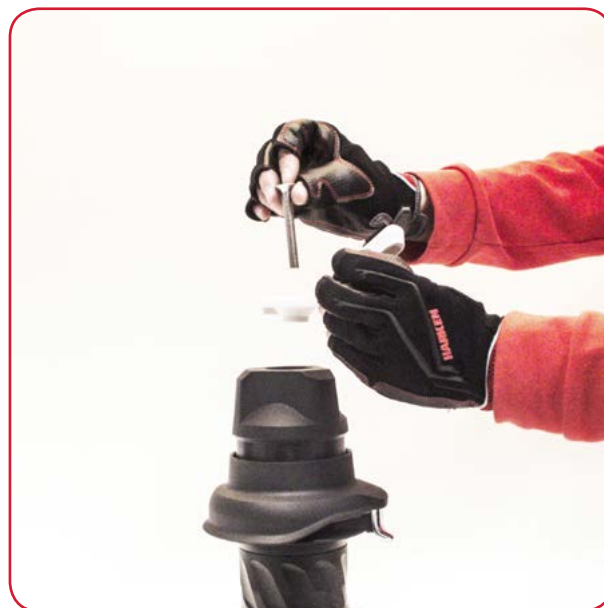
2. Position the control level using the screw supplied with transformation kit.
