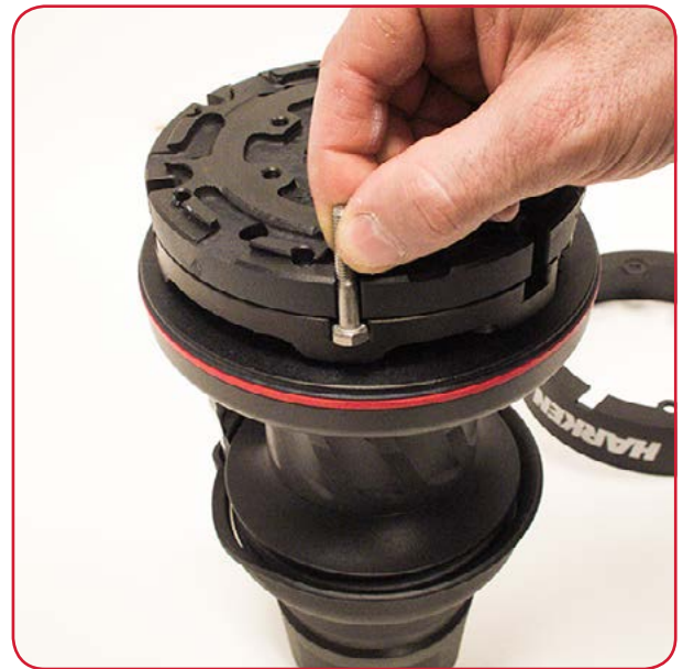
2. Take off the skirt and position the 5 M6 hexagonal headed bolts in their holes
