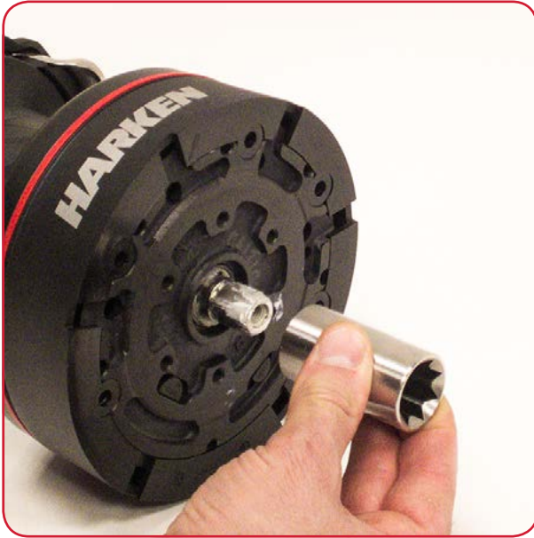
4. Position the handle socket on the shaft.
