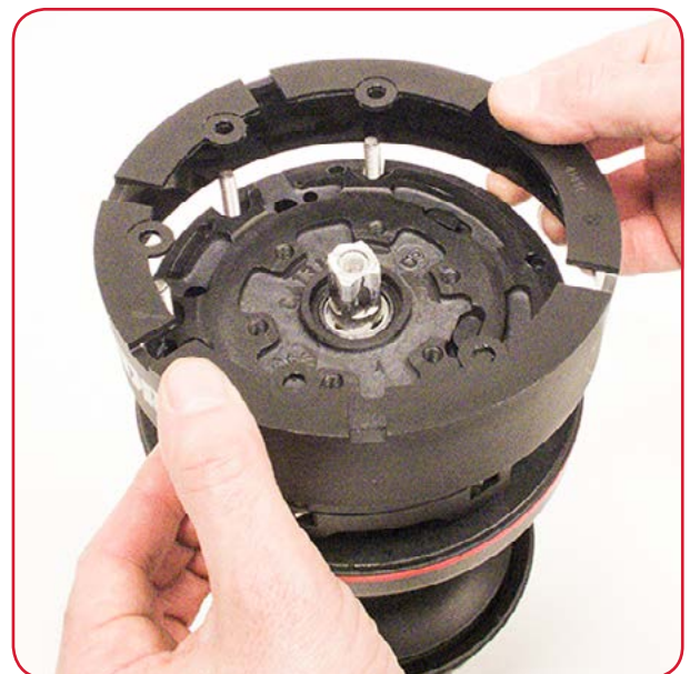
3. Reposition the skirt in housing and press down it to position correctly.
