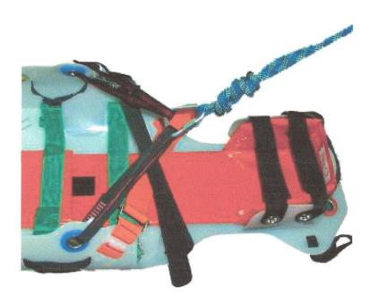
The Preferred method of attaching to the Mid Haul points for both Hauling and Security lines. Never attach a Haul or Security line into one side only.
