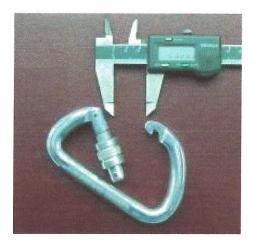
Use only karabiners with a gate opening of greater than 20mm. Using smaller karabiners will result in damage to the edge of the stretcher skin.
