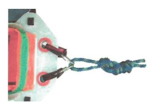
The Preferred method of attaching a Haul line to the Vertical Haul point. Never attach a Vertical Haul line to one side only.
